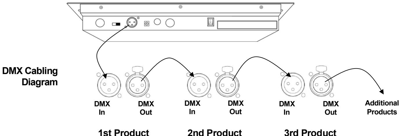
**D-Fi™ Communication** D-Fi™ communication can be used alone, or in combination with DMX cabling. Products that are D-Fi™ compatible receive D-Fi™ signal directly from the Obey™ 40 D-Fi 2.4, and products that require DMX cabling can be connected to D-Fi™ distribution products, such as D-Fi™ Hub and D-Fi™ Stream 6 which receive the D-Fi™ signal and send it out via DMX cables.
