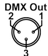
All Chauvet lights use a negative pin 2 and positive pin 3, so the polarity switch should be set as shown above and in [Back Panel View](#) (towards the DMX Control Out port). Other manufacturer's products might be different. See the individual product's User Manual for specific information
