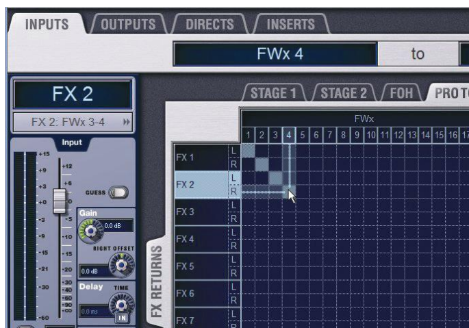
Patching FWx channels to D-Show FX Returns for playback
