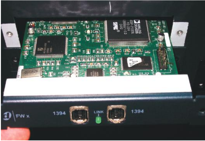
Installing the FWx card in the back of the Mix Rack
