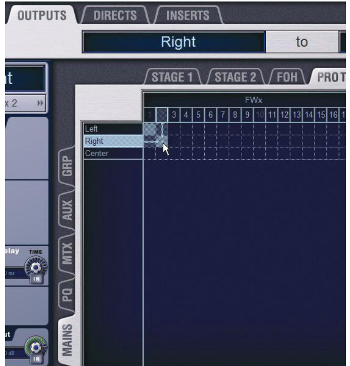
Routing the Mains bus to FWx channels for recording
