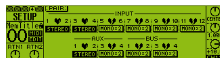
Fader grouping and channel stereo pairing functions let you control two or more channel levels by moving only a single fader in the group or pair.
