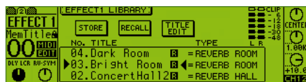
The 2 onboard professional effects processors include 42 preset programs in the Effects Library which you can freely edit and then store in 57 user programs.
