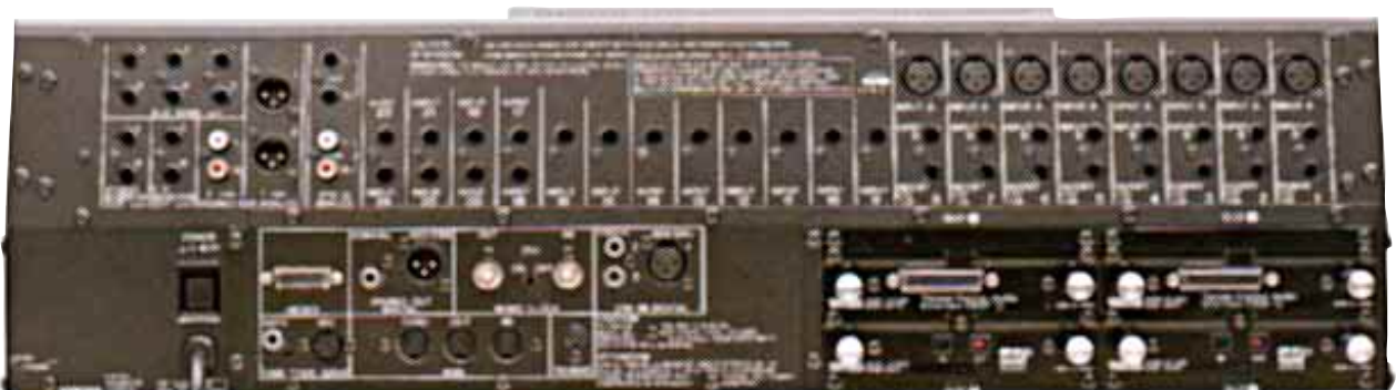
Rear panel of 02R shown with the optional TASCAM & ADAT Interface Cards installed.
